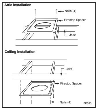
Fig. 19 Installing firestop spacer.
